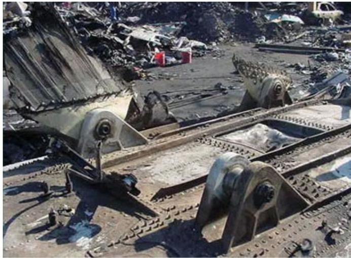
*A300 Carbon Fiber Vertical Stabilizer Failure*
