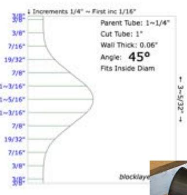
parent tube, the cut tubes wall thickness, and the angle of attachment. In this example I have had the computer calculate the cutting path based on the input parameters shown above. The output is a cutting path printed at 100% on your printer, cut out and wrapped around the cut tube. It shows the exact path to follow. If you are careful and mark the cut path with a marker you can reuse the template many times.
