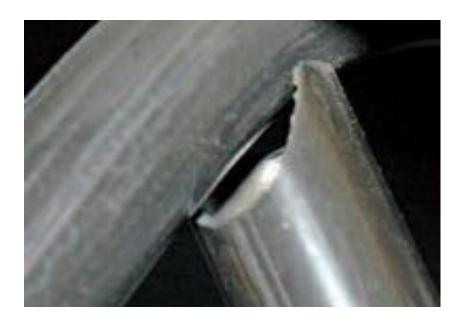
require a somewhat better fit that this, so a good tool to smooth and shape the edges of the coping would be a flap wheel on your grinder. All of this takes some time and a little skill to get a good fit up. This type of notching works best when the two pieces of tubing interface between 90 and 45 degrees. Difficulties increase when you start
